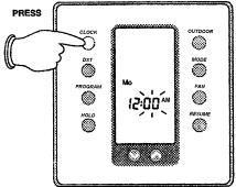
Step 2: Press the CLOCK button again and "12:" (hours) and "AM" or "PM" will flash. Use the DECREASE or INCREASE button to change the flashing symbol to the current hour making sure the hour has the proper AM or PM designation.
