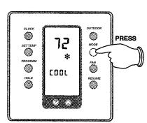
Step 1: Press and release the MODE button until the word "COOL" and the " cooling symbol appear on display.
