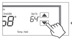
**Press** ▲ or ▼ to adjust the end time of the hold. If end time is not adjusted, the Temporary Hold will end at the start of the next event.
