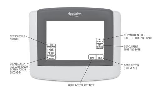
NOTES: BACKLIGHT IS ACTIVATED WITH FIRST BUTTON PRESS AND AUTOMATICALLY TURNS OFF.
