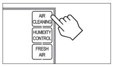
If installed, air cleaning can operate in five different modes. Air cleaning will activate the fan for the purpose of air cleaning.
