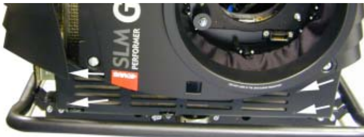
Image A-4 Dust filter removal
