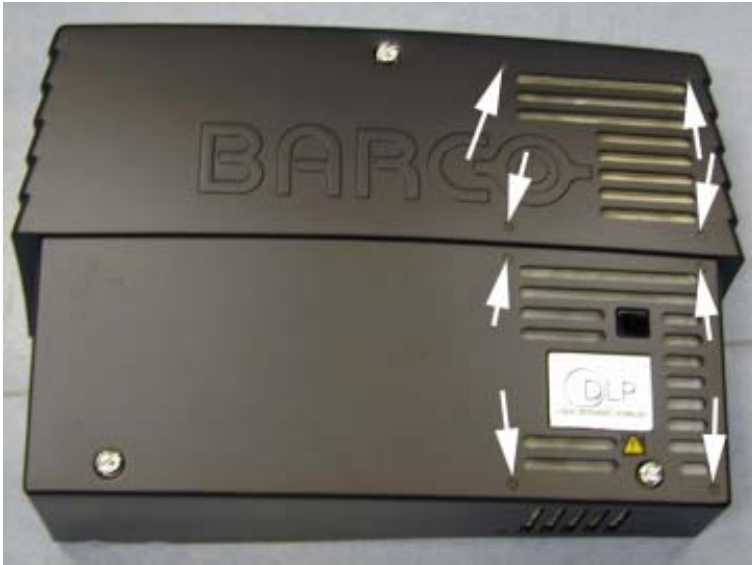
Image A-7 Dust filter removal
