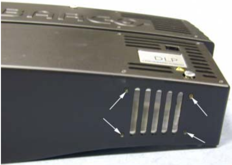
Image A-8 Dust filter removal
