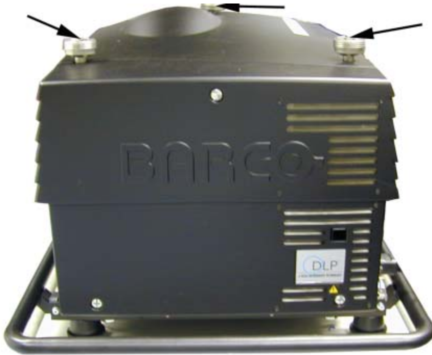
Image A-1 Removing stacking sockets
