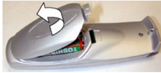
Image 2-5 Battery cover removal
