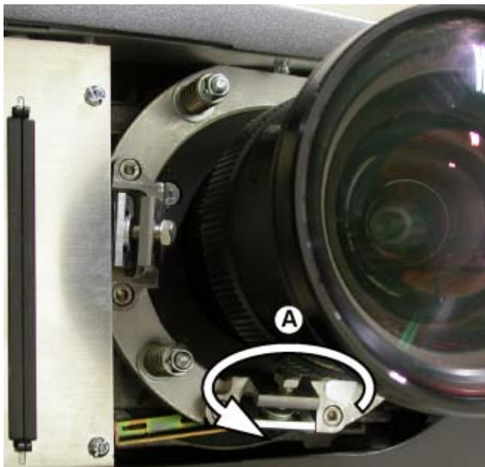
Image B-3 Turn bolt A counterclockwise to tilt the lens from top to bottom.
