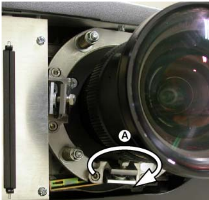
Image B-5 Turn bolt A clockwise to tilt the lens from bottom to top.
