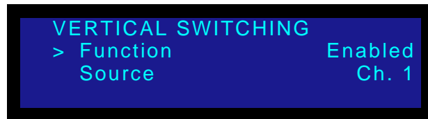
Figure 4-15. MatrixPRO Vertical Switching Menu (sample)
