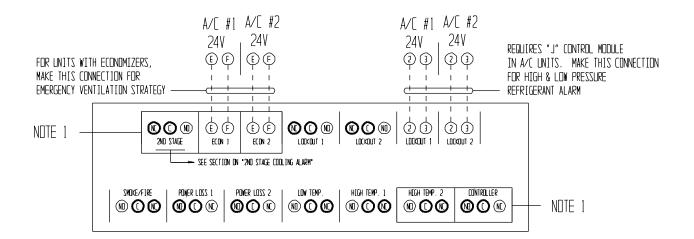
USE SHADED TERMINALS FOR DESIGNATED ALARMS AS DESIRED. SOME RELAYS ARE REVERSE ACTIVATED TO ACHIEVE "NC" OPEN-ON-ALARM SEQUENCE. EACH CAN BE USED INDIVIDUALLY IF THERE ARE ENDUGH BUILDING ALARM POINTS AVAILABLE OR CAN BE ARRANGED INTO SMALLER GROUPS OR EVEN A SINGLE GROUP SO THAT ALL ALARM CAPABILITIES CAN BE UTILIZED. FOR "NC" OPEN-ON-ALARM STRATEGY MULTIPLE ALARMS IN A GROUP ARE WIRED IN SERIES.
