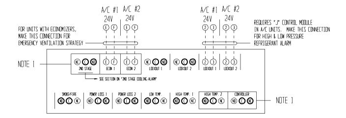
LISE SHADED • TERMINALS FOR DESIGNATED ALARMS AS DESIRED. SOME RELAYS ARE REVERSE ACTIVATED TO ACHIEVE "NO" CLOSE-ON-ALARM SEQUENCE. EACH CAN BE USED INDIVIDUALLY IF THERE ARE ENDUGH BUILDING ALARM POINTS AVAILABLE OR CAN BE ARRANGED INTO SMALLER GROUPS OR EVEN A SINGLE GROUP SO THAT ALL ALARM CAPABILITIES CAN BE LITTLIZED. FOR "NO" CLOSE-ON-ALARM STRATEGY MULTIPLE ALARMS IN A GROUP ARE WIRED IN PARALLEL.
