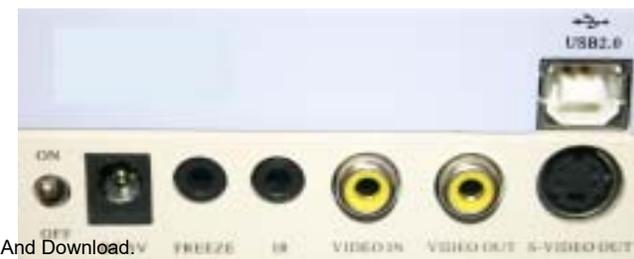
**Notes:** Cameras that start with PA or NT, you will need to press the freeze button to activate the camera's LED's. This will turn the camera on. Then you will be able to see an image from the camera.
