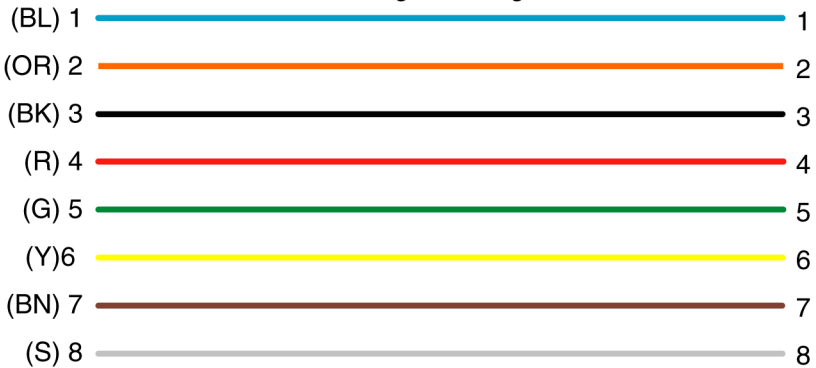
RJ-45 to RJ-45 Straight-Through
