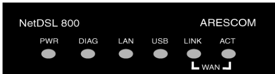
Figure 2.2 Front Panel Interfaces for NetDSL
