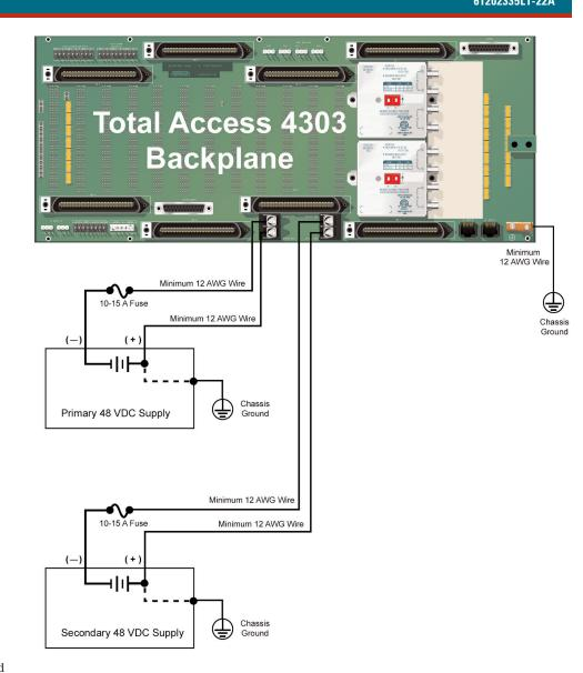
Note: Only one of the above supplies is necessary for proper Operation.
