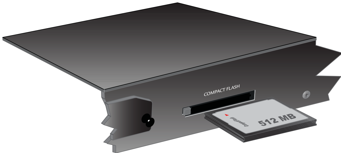
Figure 41. CompactFlash Card Installation
