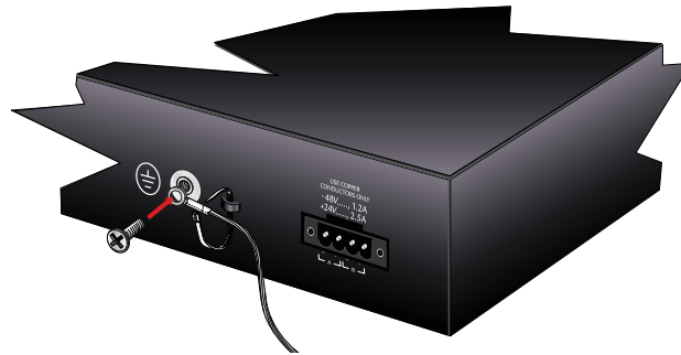
Figure 37. Grounding the NetVanta 1224STR (DC)
