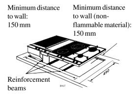
It is not necessary to attach the reinforcement beam to the work top surface, as it is held in place by a specially designed moulding, which is incorporated in the hob units flanges.
