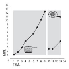
You can get a necessary heat setting in a shorter time if you activate the Automatic Heat Up function. This function sets the highest heat setting for some time (see the illustration), and then decreases to the necessary heat setting.
