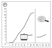
You can get a necessary heat setting in a shorter time if you activate the Automatic Heat Up function. This function sets the highest heat setting for some time (see the illustration), and then decreases to the necessary heat setting.
