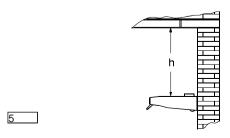
● Set the chimney according to the measured height and stop its run with the two fixing screws 2,9x6,5 mm supplied (fig. 6).
