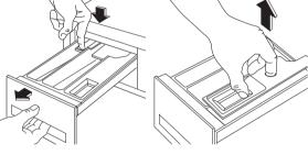
tap. To remove the drawer from the machine, press the button in the rear left-hand corner.
