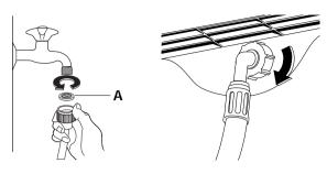
The other end of the inlet hose which connects to the machine can be turned in any direction. Simply loosen the fitting, rotate the hose and retighten the fitting, making sure there are no water leaks.
