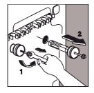
Use a 10 mm spanner to remove the two screws and spacers at the back.
