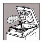
Open the washing machine lid and remove the immobilization packing and plastic films. Close the lid.
