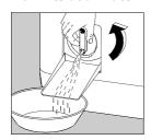
Put a receptacle under the drain. Turn the cap in the anti-clockwise direction until it is vertical to release residual water.
