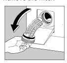
Unscrew the cap all the way and take it off. Clean it tho-roughly with running water. Put the assembly back and screw it in the clockwise direction.
