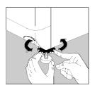
When the washing machine is stable, maintain the stand on the ground and turn the locking collar as far as possible.
