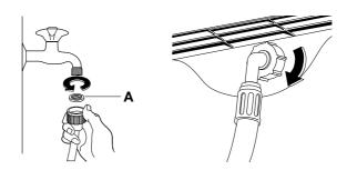
The other end of the inlet hose which connects to the machine can be turned in any direction. Simply loosen the fitting, rotate the hose and retighten the fitting, making sure there are no water leaks.
