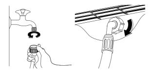
The other end of the inlet hose which connects to the machine can be turned in any direction. Simply loosen the fitting, rotate the hose and retighten the fitting, making sure there are no water leaks.
