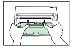
6 Push the lock lever (L) back into its locked position (away from you).
