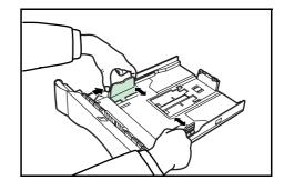
4 Set the paper in the cassette so that the leading edge is aligned against the paper stopper, but making sure that none of the paper gets caught on the overhanging tabs.
