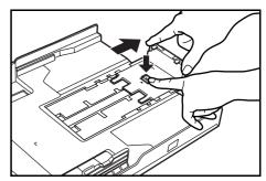
2 Remove the stopper extension lock from the paper stopper.
