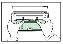
**9** Push the lock lever back into its locked position (away from you).
