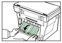
2 Perform the standard copying or printing procedure. Finished copies or printouts will be output onto the face-up tray.
