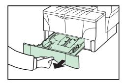
**Important** When pulling the cassette out of the machine, be sure to support it so that it doesn't fall out suddenly.
