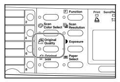
5 Press the ▲ key or the ▼ key to select the desired mode and press the Enter key. The message display returns to the basic screen.
