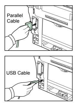
**3** Connect the other end of the printer cable to the parallel interface connector or USB interface connector on your computer.
