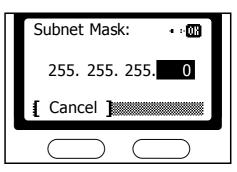
4 When you finish making all of the network setting, press the right **select** key. The message display returns to the basic screen.
