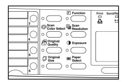
3 Press the **Paper Select** key to select paper feed location, and press the **Enter** key. The message display returns to the basic screen.
