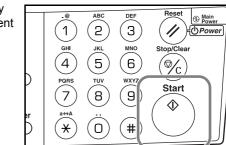
11 Press the **Start** key. Scanning will begin immediately once the **Start** key will light. The scanned image is sent to the entered destination e-mail address as an attachment. The image is named as doc.pdf (default).
