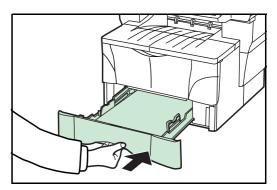
6 Register the paper size loaded in the corresponding cassette above by using the operation panel. For detail, refer to *Chapter 5* in *Advanced Operation Guide*, *Selecting Paper Size and Media Type*.
