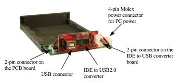
**Note:** The Hot Swap feature for the above configurations is enabled by the connection of the power cable connected to the 2-pin connector on the PCB board on the cradle and the 2-pin connector on the IDE to SATA or IDE to USB converter boards. With this feature you can remove the Jupiter Cipher ExDrive from the cradle without shutting down the system.
