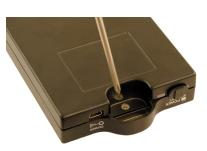
**Step 1**Separate the top from the bottom cover of the drive enclosure by loosening the screw as shown on the photo.
