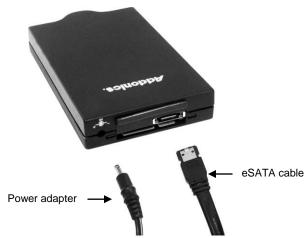
**Step 1:** Connect the eSATA cable to the eSATA port at the back of the enclosure. The other end of the cable connects to the eSATA port on the USB2.0 to eSATA adapter. Plug the adapter to a USB port on your system.
