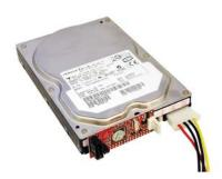
At the other end of the Y-power cable is the 4-pin floppy power connector which you connect to the converter. Now connect the SATA cable to the SATA port on the converter.
