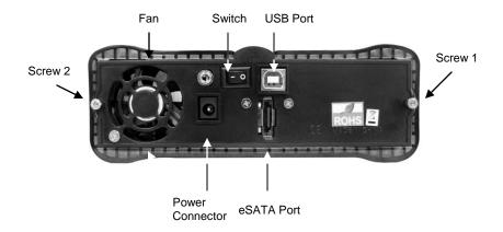
Removing the front panel
