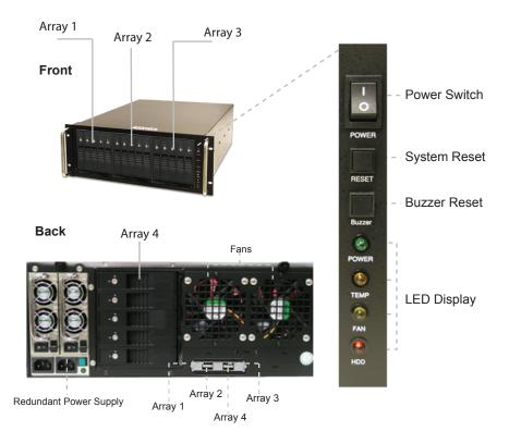
**Power Switch:** This is the switch to power on devices connected to the power supply. The power LED will light up to indicate power is supplied. Note: The main power switch located at the back of the enclosure must be turned on first.
