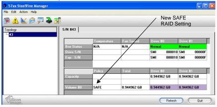
Note: The steps for creating BIG or FAST RAID set would be similar with the steps on creating SAFE RAID set. Only select the correct switch setting.
