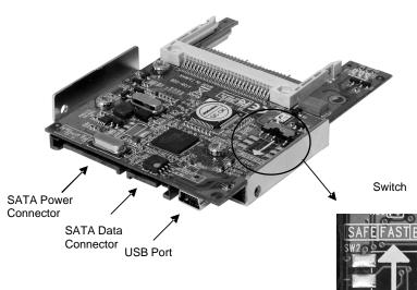
**Note:** The default setting for the RAID setting is BIG. The switch has 3 settings. You slide the switch from left to right to change RAID setting.
