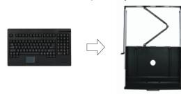
2. Pull the keyboard wire through the hole until to the back of the keyboard drawer.
