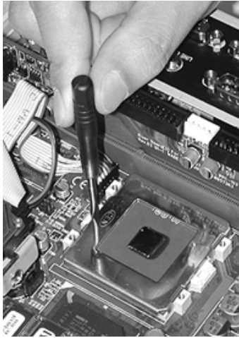
Figure 3-5: Insert screw driver into the hole
