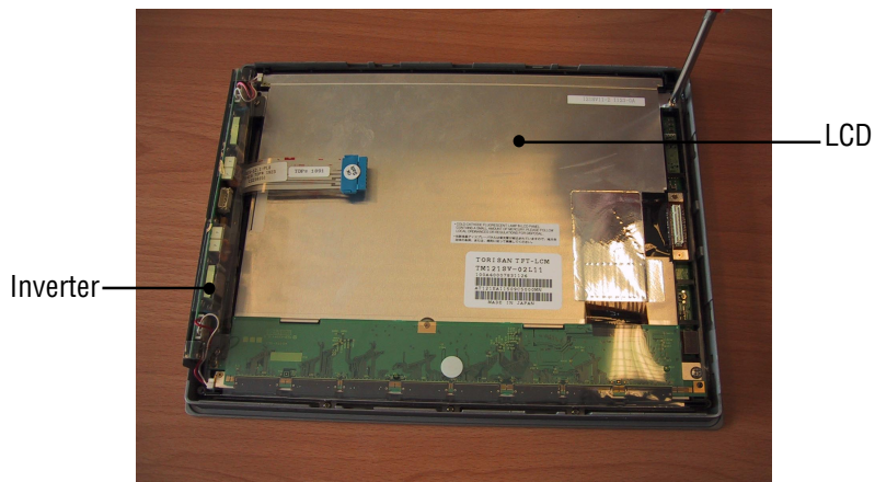
Figure B-5: Remove the inverter and LCD
