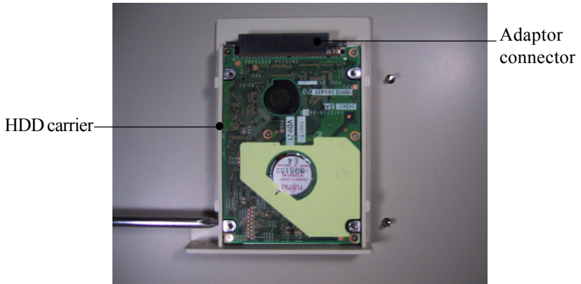
Figure 3-1: Install the HDD on the HDD carrier
