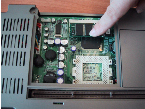
Figure 3-9: Installing the memory module
