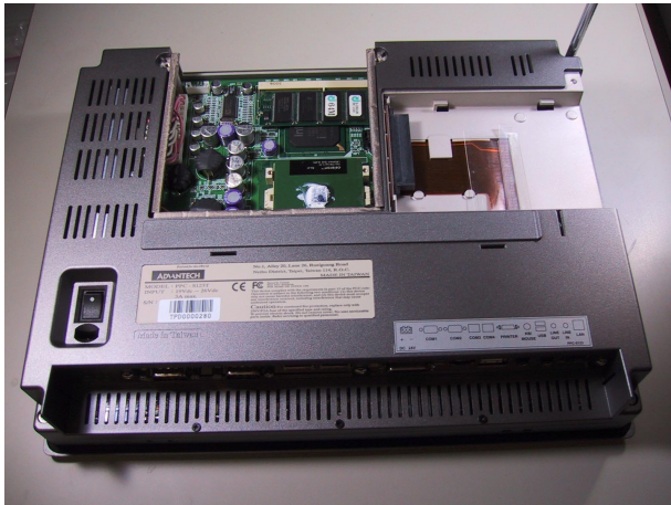
Figure B-3: Remove the seven screws on the rear panel
