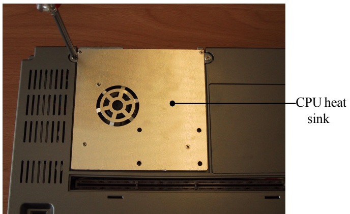
Figure 3-3: Detach the CPU heat sink
