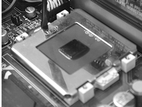
Figure 3-4: Place CPU push cover over CPU
