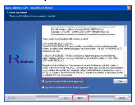
Step1.1: In Windows XP, You can choose to configure the adapter through the **Microsoft**Zero Configuration Tool or the Ralink Configuration Tool. It is recommended to choose the Ralink Configuration Tool for the adapter. Click Next to continue.
