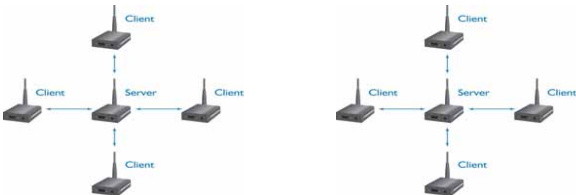
Figure 9- Multiple Networks of Point-to-Multipoint CL4424s
