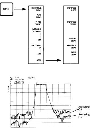
CENTER 32.265975000 GHz SPAN 15.000000000 GHz Probably the most frequently used feature to improve the data presentation is averaging. Press RESPONSE (MENU), then [AVERAGING ON/restart]. The active function is now the averaging factor applied to the measurement.
