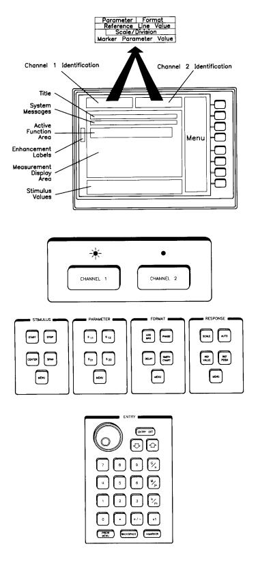
**CRT Display.** The front panel of the network analyzer is relatively simple. It is shown in full by the foldout at the end of this document. First, there is the CRT which presents the measurement results. This illustration shows the general areas for the measurement trace and for the various annotations which communicate to the operator.
