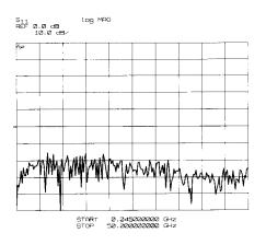
Pressing the green (USER PRESET) key initializes all HP 8510 internal functions, then recalls Instrument State 8. An instrument preset command is not sent to other instruments connected to the HP 8510 system bus. Unless the user has changed the contents of Instrument State 8, the CRT will appear as shown here, with the current S11 measurement displayed in the logarithmic magnitude format. The appearance of the trace will depend upon the actual connection to PORT 1 of the test set.
