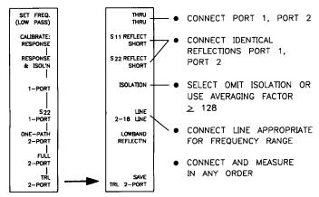
TRL 2-PORT calibration type uses multiple measurements of the thru connection, identical reflection standards at each port, and a transmission line of appropriate length and impedance to measure the error terms. If proper standards are available, this is the preferred technique due to fewer connections required and the potential for more accurate characterization of the error terms. More details of this calibration procedure are contained in other documentation supplied with the HP 8510 system.
