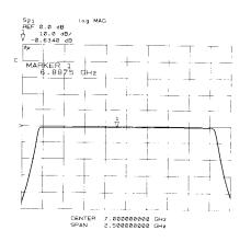
Calibration for insertion loss and gain sets the magnitude ratio to zero dB at all frequency points with the thru connection. After connecting the test device, a negative measured value indicates loss; a positive measured value indicates gain. This figure shows the insertion loss of a bandpass filter.
