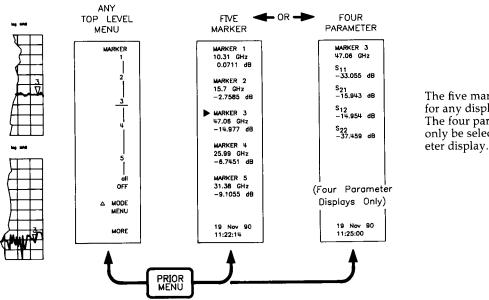
The five marker list can be selected for any display mode. The four parameter marker list can only be selected with a four parameter display.
