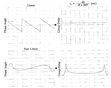
**Group Delay.** The phase linearity of many devices is specified in terms of group or envelope delay. This is especially true of telecommunications components and systems. After calibration, select (DELAY) to view the group delay of the DUT.
