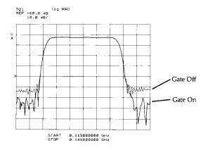
Time domain analysis also lets you remove individual parts of the time domain response to see the effect of potential design changes. We do this by mathematically "gating" out the undesired responses. In this example we see the effect of removing the leakage and triple travel responses using the gating feature. Press
