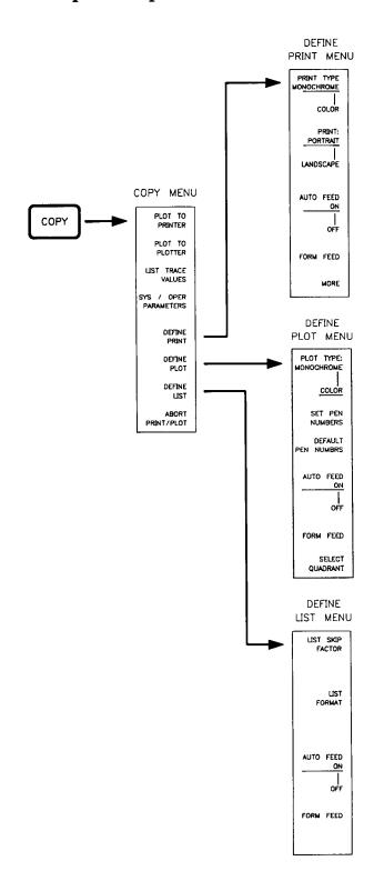
Measurement results can be output to a graphics printer, digital plotter, or a line printer using using selections in the  $(\overline{\text{COPY}})$  menu structure. The HP 8510C adds two RS-232 ports for connection of hardcopy output devices. Moving the output devices from the 8510 system bus to the RS-232 ports may improve measurement throughput because since the RS-232 ports are fully buffered, the measurement can continue while the plot is being produced.
