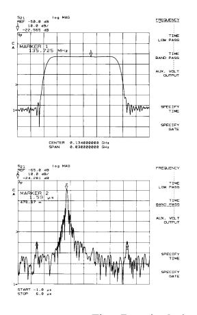
Now connect the SAW filter. These figures show the frequency domain response and the time domain response of this device. Note the three components of the transmission time domain response: RF leakage, at near zero time, the main travel path through the device (about 1.6 microseconds), and the "triple travel" path (about 4.5 microseconds travel time). Each of these signal paths is shown in the measurement.
