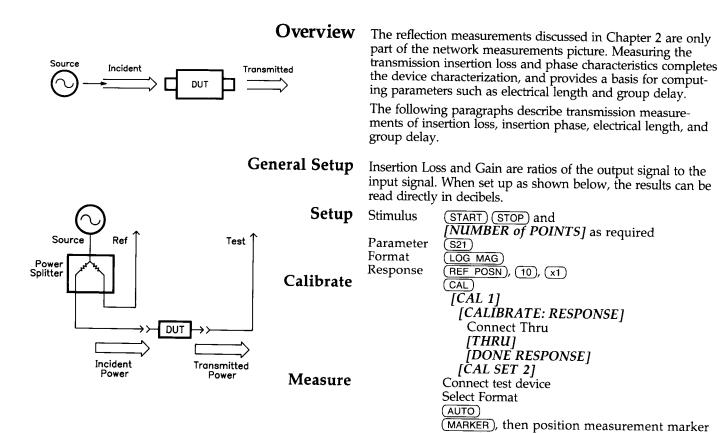
Measuring Insertion Loss and Gain Calib
