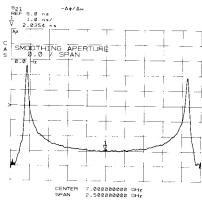
After selecting the minimum aperture, you may increase the effective aperture of the measurement using the smoothing function. Press RESPONSE (MENU), then [SMOOTHING ON]. Use the knob or numeric entry to set the effective aperture. Note that increasing the aperture smooths the group delay trace, removing fine grain variations form the response. This is why, when comparing group delay measurements, the aperture must be specified.
