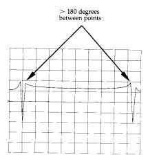
**Group Delay Aperture.** The minimum aperture is the frequency step between the phase measurements. You must choose this aperture when you set the frequency range and number of points so that there is no more that 180 degrees of phase shift between any of the frequency points. If there is more than 180 degrees of phase shift, the group delay trace will show a sudden discontinuity.
