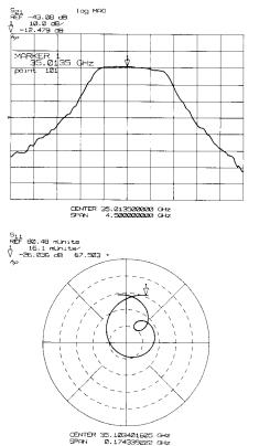
Twelve different display formats provide a comprehensive selection of useful presentations. The keys in the FORMAT block and displayed by FORMAT (MENU) also select the marker units shown by the active marker. This list shows the trace value and marker units for each of the standard format selections. Examples of how these formats are used for various reflection and transmission measurements are discussed in later chapters.
