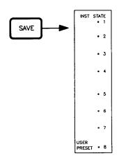
Press (SAVE), then select one of the eight instrument state registers to save the current instrument state. All control settings, including the P/F/R limited instrument state for each channel, are saved. Please note that the contents of the cal set are not saved, only the reference to any cal sets that are turned on.
