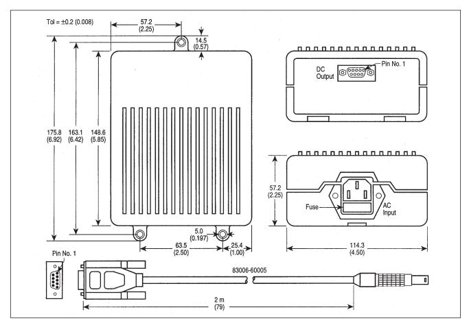
The Agilent 87421A power supply provides the dc power needed to bias the 83006A, 83017A, and 83018A. The power supply comes with a 2 meter long cable to allow easy connection between the amplifier and the power supply. Dimensions in millimeters and (inches).
