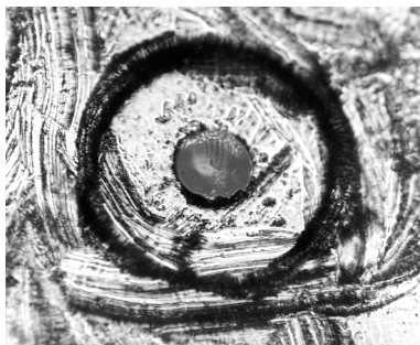
Figure 1-6. Damage from improper cleaning.
