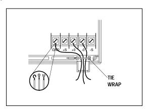
Route the wires out of the bottom of the connector as shown in the figure above. Use the tie-wrap supplied with the connector to secure the wires to the connector.
