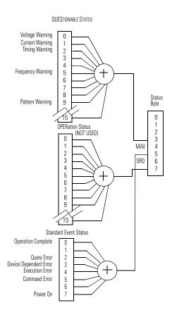
The instrument has a status reporting system conforming to IEEE 488.2 and SCPI. The above figure shows the status groups available in the instrument.
