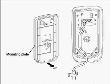
Cut out the knockout at the bottom of the mounting plate and wire the required wires to the main unit side.
