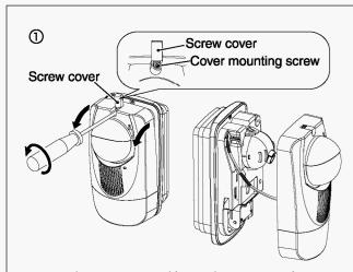
Remove the screw cover and loosen the cover mounting screw. Pull the top of the two sides of the main unit cover toward you and remove the main unit cover.
