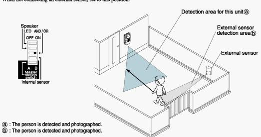
\*When connecting an external sensor, install it somewhere that the camera on this unit can photograph anyone who enters that external sensor's detection area. \*When not connecting an external sensor, use "OR mode".
