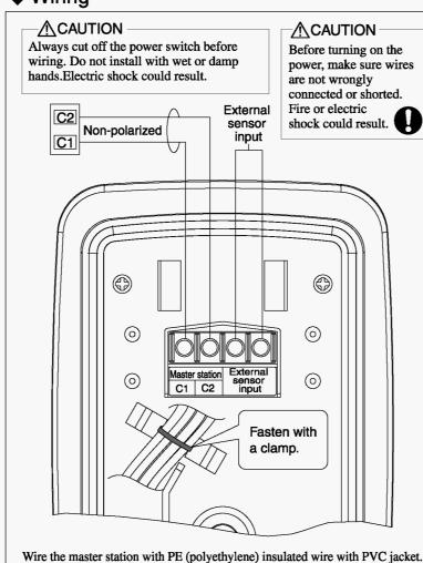
Single core wire Ø 0.65 mm Ø 0.9 mm Ø 1.2 mm Distance 50 meters max. 100 meters max. 100 meters max.
