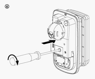
Mount the unit onto the frame, then tighten down the lock Next, adjust the camera and sensor.
