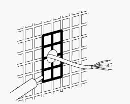
When mounting on an outside wall with a large gap or on an uneven surface, such as tiles, fill in the mounting surface grooves and gaps with caulk.
