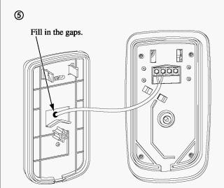
Connect the necessary wires. X See the "Wiring diagram". After that, fill in the gap at the wiring hole section.
