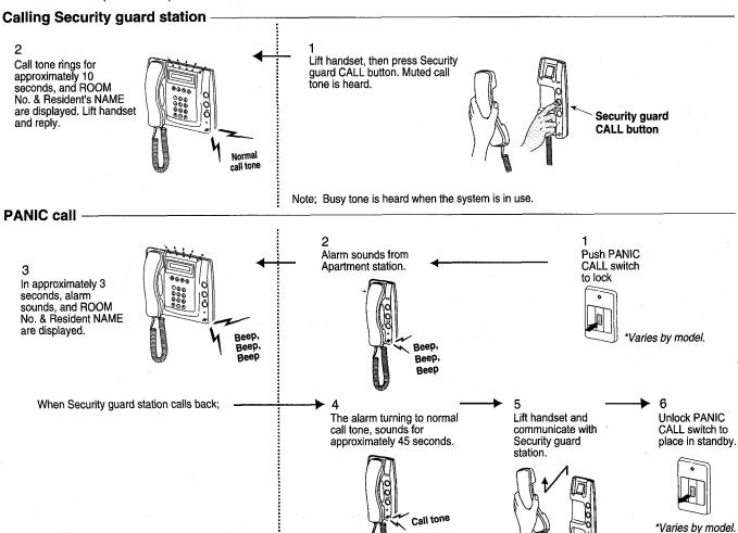
Notes; Line-off trouble alarm will be activated when the wires are off at PANIC CALL button. The alarm will sound even when the station is busy. (at the HIGH volume regardless of the setting)
