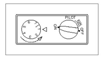
CAUTION: Do not try to adjust heating levels by using the manual shutoff valve.
