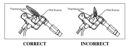
If pilot flame pattern is incorrect as shown above, turn heater off and refer to troubleshooting guide.
