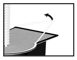
Step 2 Remove the wax paper from the gasket. Step 3 Insert unit into pre-cut hole.
