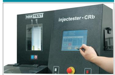
Easy to use touch panel provides a fast operation while the user interface menu's help and guide the operator at every step of the test from starting the test to printing the report. Well designed user interface prevents the user from losing time between menu pages
