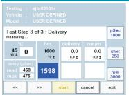
Injection delay is measured in usec. Delay is characteristic for each model of injector and also provides information about the consistancy of its operation. Even when running at very high speed, the delay can be measured with accuracy.
