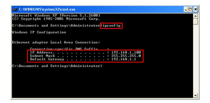
Step 3 Write down the values for the IP Address, Subnet Mask, and Default Gateway on a piece of paper.
