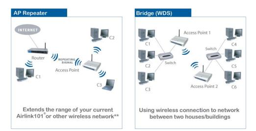
If you want to use the AP431W as an Access Point with minimal configuration, just connect it to your existing router or switch with a Cat. 5 network cable and then power it on. The Access Point is ready to use with its default settings:
