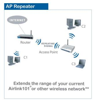
**Note:** The repeater mode may not be compatible with all routers due to the lack of a standard protocol for repeater mode.
