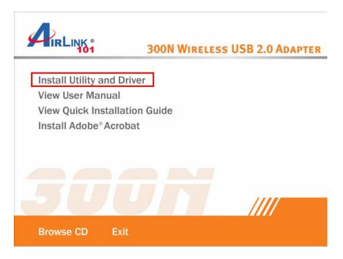
**Note:** If the Autorun screen doesn't appear automatically, or if you get a blank white screen, go to **Start**, **Run**, and type **D:\Utility\Setup.exe** (where **D** is the letter of your CD drive) and click **OK**.
