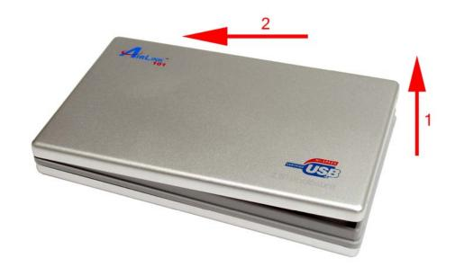
**Step 3** Remove the bottom cover in the same manner. If you find it hard to lift the plastic holder, press it slightly inward.
