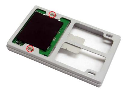
*Caution:* Be sure to remove the circuit board from the plastic holder before attaching the hard drive; otherwise, the hard drive's IDE pins may be damaged.
