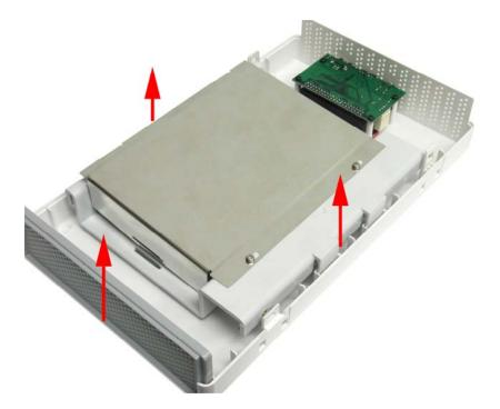
**Step 5** Place the CD/DVD drive with the drive's top facing up and then connect the IDE cable and the power cord to the drive. Make sure the CD/DVD drive you are installing is set to "**Master**" (refer to the jumper setting information printed on your CD/DVD drive).
