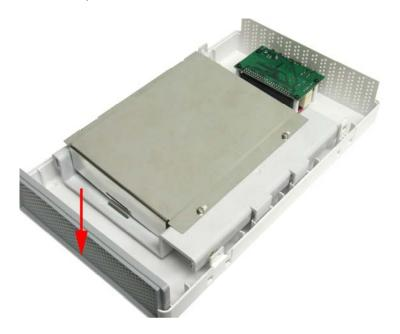
Step 10 Replace the top cover and re-secure the screws removed in Step 1.
