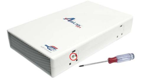
**Step 3** Remove the top cover. If you find it hard to open the cover, use the screwdriver to slightly push the locking tab inside.
