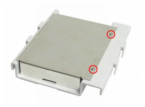
**Step 8** Connect the IDE cable and power cord to the hard drive and then hook plate B back to the enclosure. (Be sure to apply enough force to properly secure the drive).
