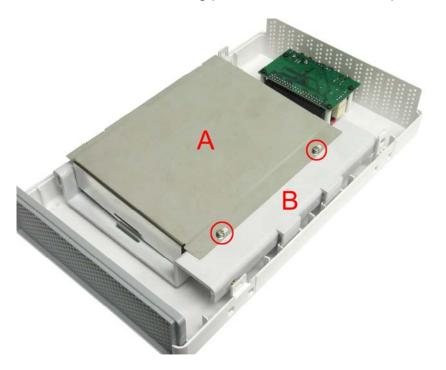
**Step 5** Remove plate B from the enclosure box and place the hard drive as shown below. Make sure the hard drive you are installing is set to "**Master**" (refer to the jumper setting information printed on your hard drive).
