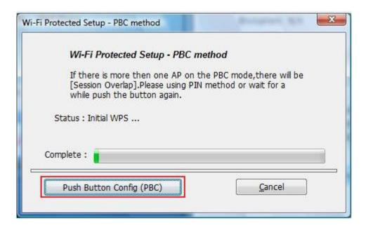
**Step 4.6.2b** Push the Easy Setup Button (WPS button) on the router, and it will start the handshake with wireless adapter. The connection will be built up in couple minutes.
