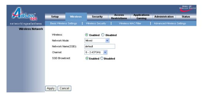
Wireless: Select to Enable or Disable the wireless feature of the router.
