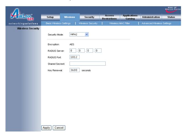
**Encryption Methods**: Select either **TKIP** or **AES** as the encryption method. (WPA2 uses AES only).
