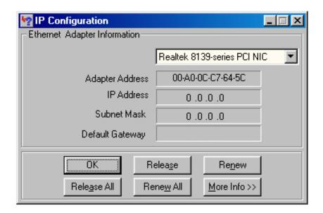
**Step 8** After your IP address is released, click **Renew**. You should get an IP address of **192.168.1.x** (where **x** is a number between 2 - 254). If you don't get an IP address, reset the router by holding in the reset button at the back of the router for 10 seconds while it is ON and try **Renew** again.
