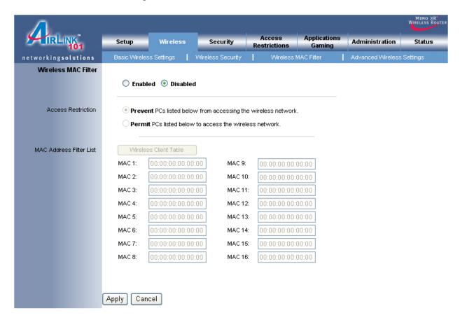
Select **Enabled** and choose whether the specified wireless clients will be prevented or permitted to access the wireless network. Enter their MAC address in the fields below and click **Apply** to save the setting.
