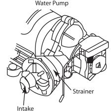
Turn Intake Counter-Clockwise to remove
