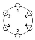
NOTE: Use a torque wrench to tighten lug nuts. Tightening by hand or with an impact wrench is not recommended.
