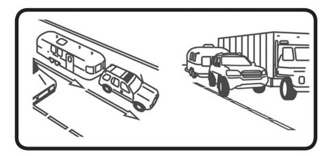
When going downhill in dry weather, down shift so that engine compression will slow the whole rig down. Take dips and depressions in the road slowly and do not resume normal driving speeds until you are sure that the trailer wheels are clear of the dip.
