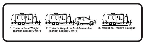
When loading heavy objects such as tools, skillets, irons, and boxes of canned goods, etc. keep them as low as possible - preferably on the floor. Try to hold additional weight behind the axle to a minimum.
