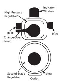
All models are equipped with an automatic gas regulator. Both tanks are connected to this regulator.
